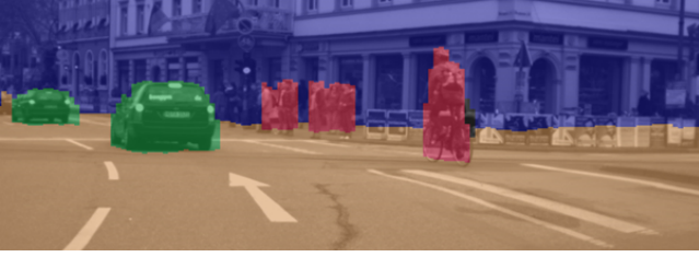
Figure 2: Semantic scene model recovered using stereo vision-based scene understanding. Different colors encode distinct semantic object classes: road surface (brown), humans (red), vehicles (green), and buildings (blue) [4].
